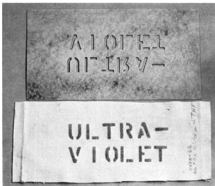
Fig. 1. Cotton cloth decorated with epoxy resin formulation described in text. Formulation applied in tetrahydrofuran solution, allowed to dry overnight, covered with stencil, exposed to AH-6 lamp for 15 min, baked 2.5 hr at 125°C, soaked in methyl ethyl ketone to remove unexposed resin. Letters in image are 1.9 cm in height.
